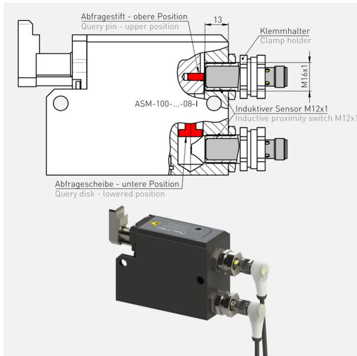
The upper and lowered position of the stop module can be queried with inductive sensors at the stop module ASM-100-...-08-I and ASMHS-100-...-08-I
