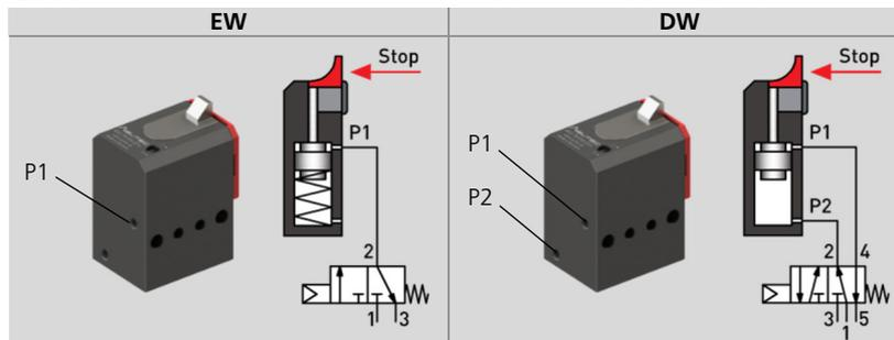
The stop modules ASU-70 are offered as single-acting variants (EW) and double acting variants (DW). For the EW-version there is only one air connection (P1) for lowering the stop module and for the DW-variant there is an additional air connection P2 for raising the stop module.
